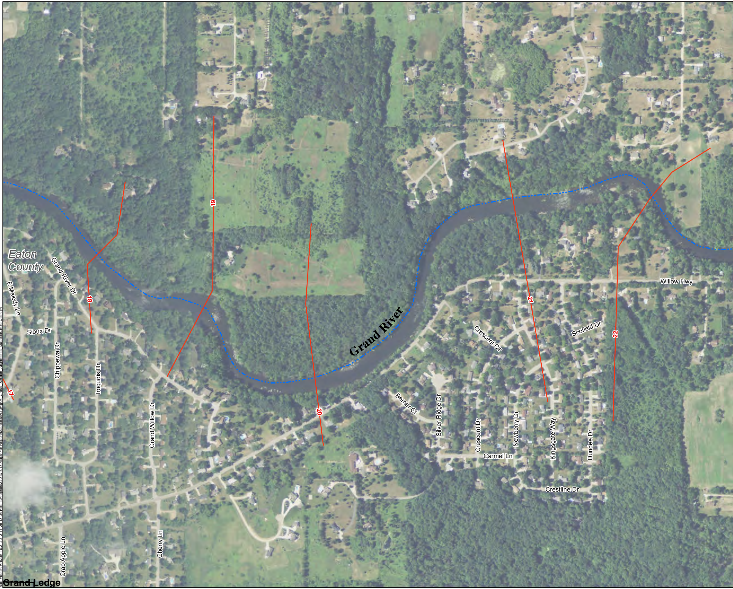
Large Figure 6 – 16 HEC-RAS CROSS SECTIONS Moores Park Dam and North Lansing Dam Break Model Lansing Board of Water and Light November 2013
