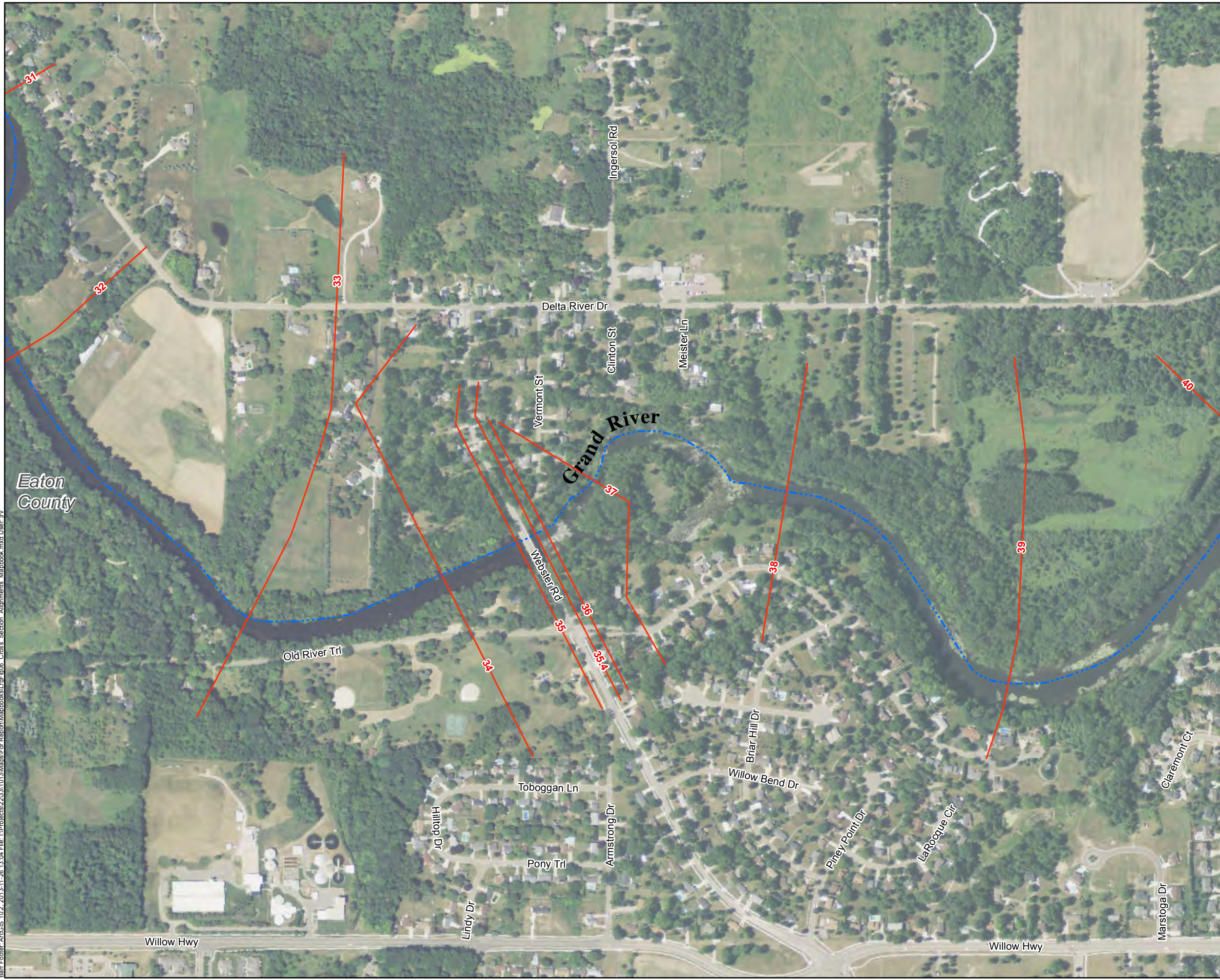
Large Figure 6 – 13 HEC-RAS CROSS SECTIONS Moores Park Dam and North Lansing Dam Break Model Lansing Board of Water and Light November 2013
