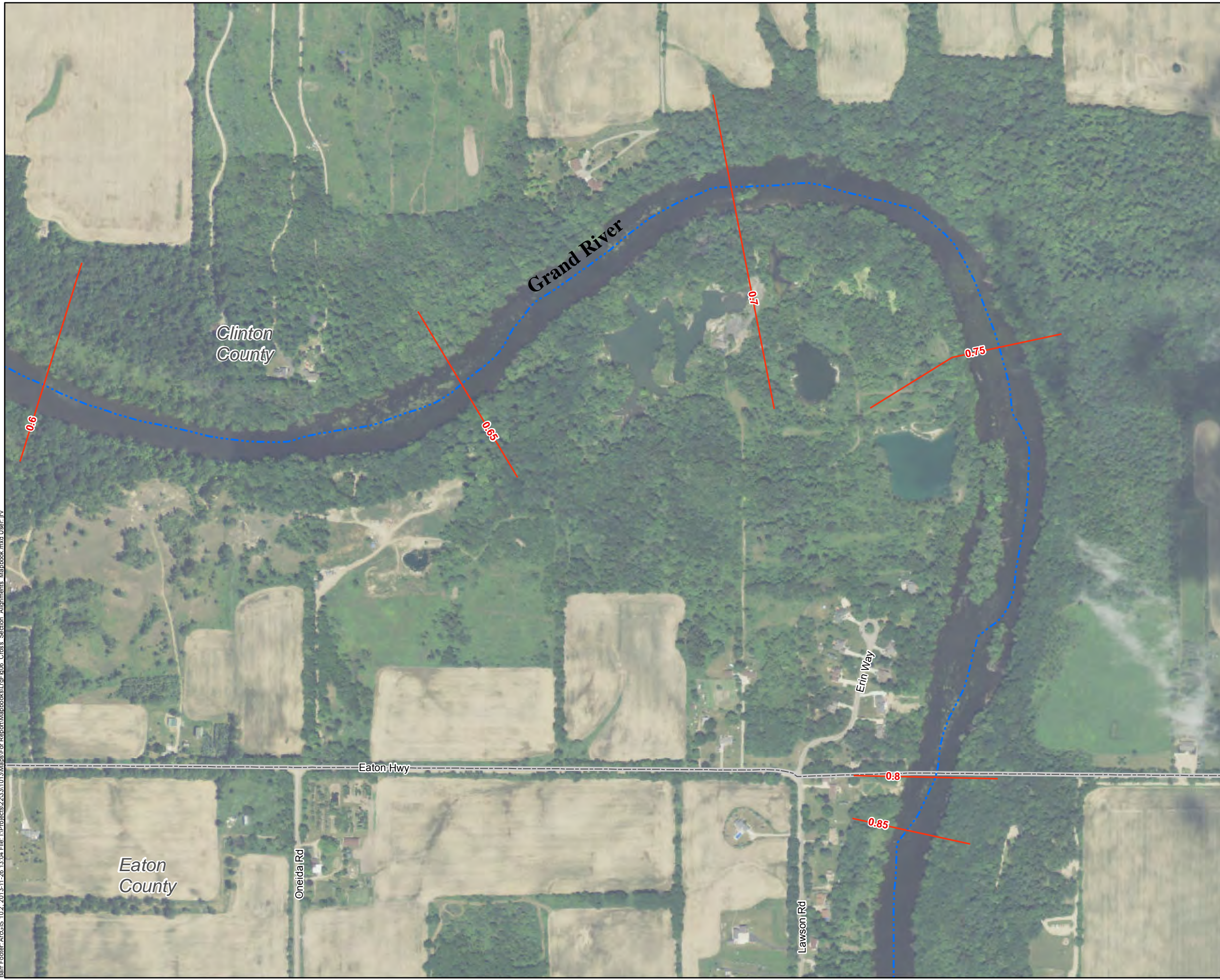
Large Figure 6 – 19 HEC-RAS CROSS SECTIONS Moores Park Dam and North Lansing Dam Break Model Lansing Board of Water and Light November 2013
