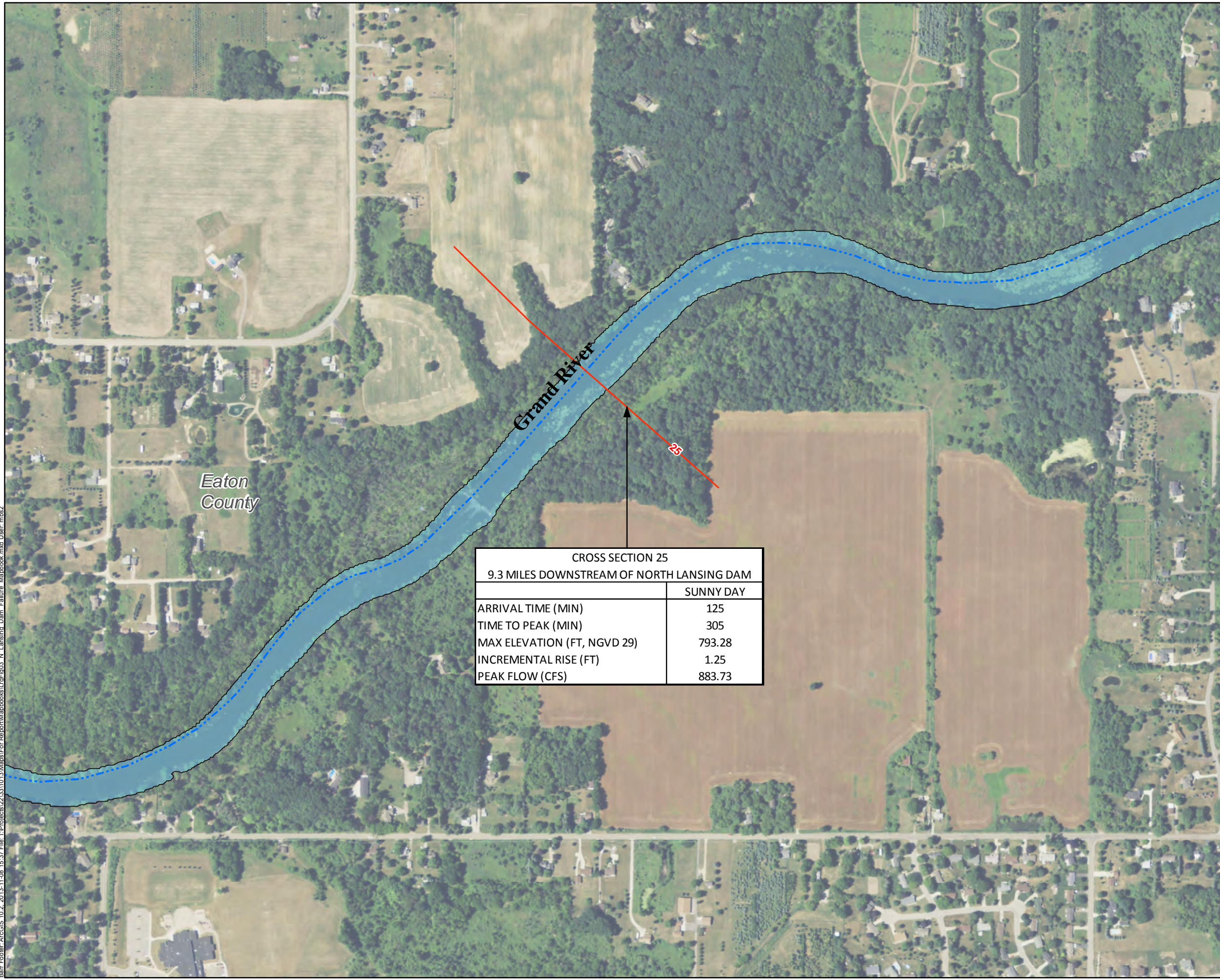
Large Figure 3 – 07 NORTH LANSING DAM FAILURE ONLY INUNDATION Moores Park Dam and North Lansing Dam Break Model Lansing Board of Water and Light November 2013
