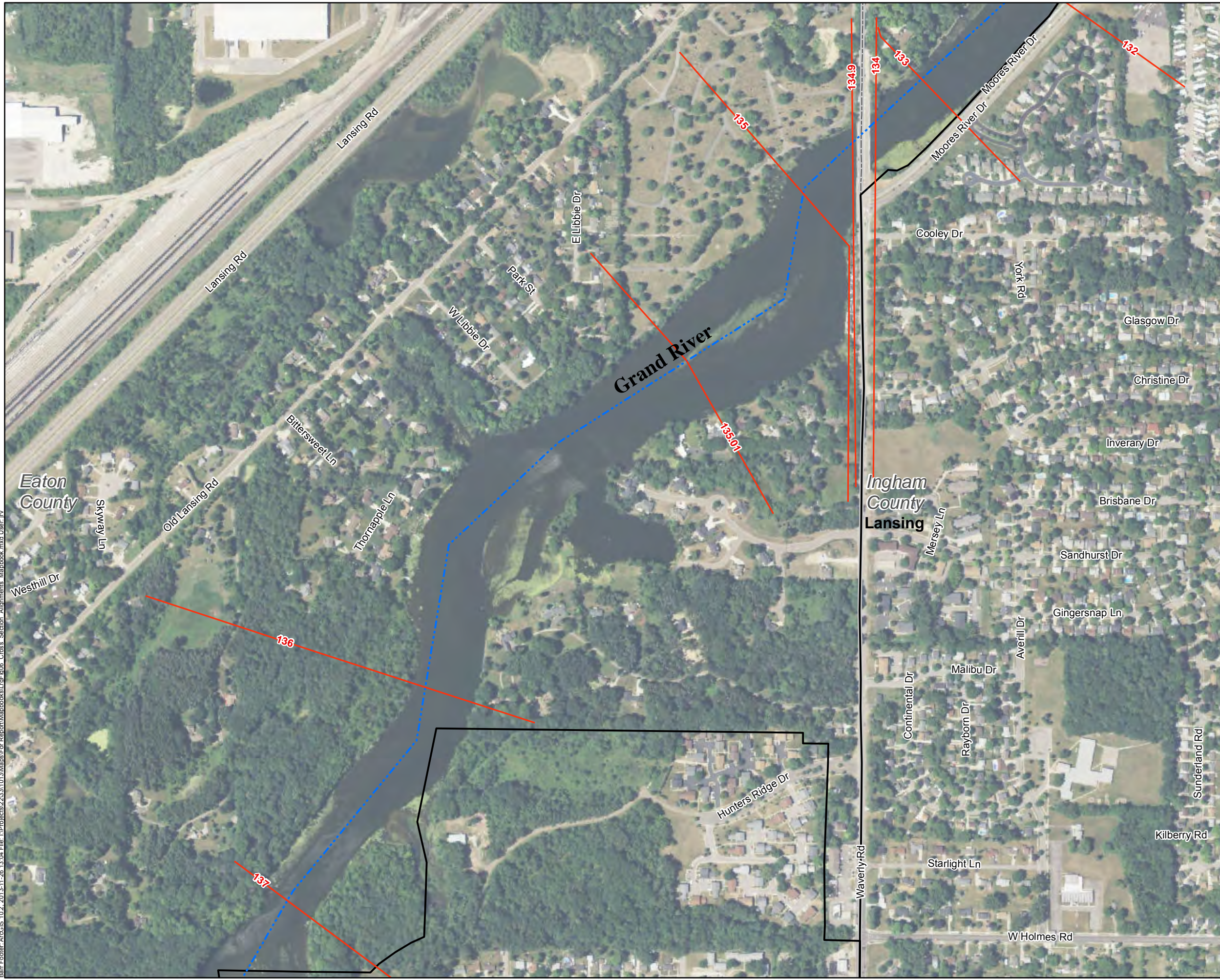
Large Figure 6 – 03 HEC-RAS CROSS SECTIONS Moores Park Dam and North Lansing Dam Break Model Lansing Board of Water and Light November 2013
