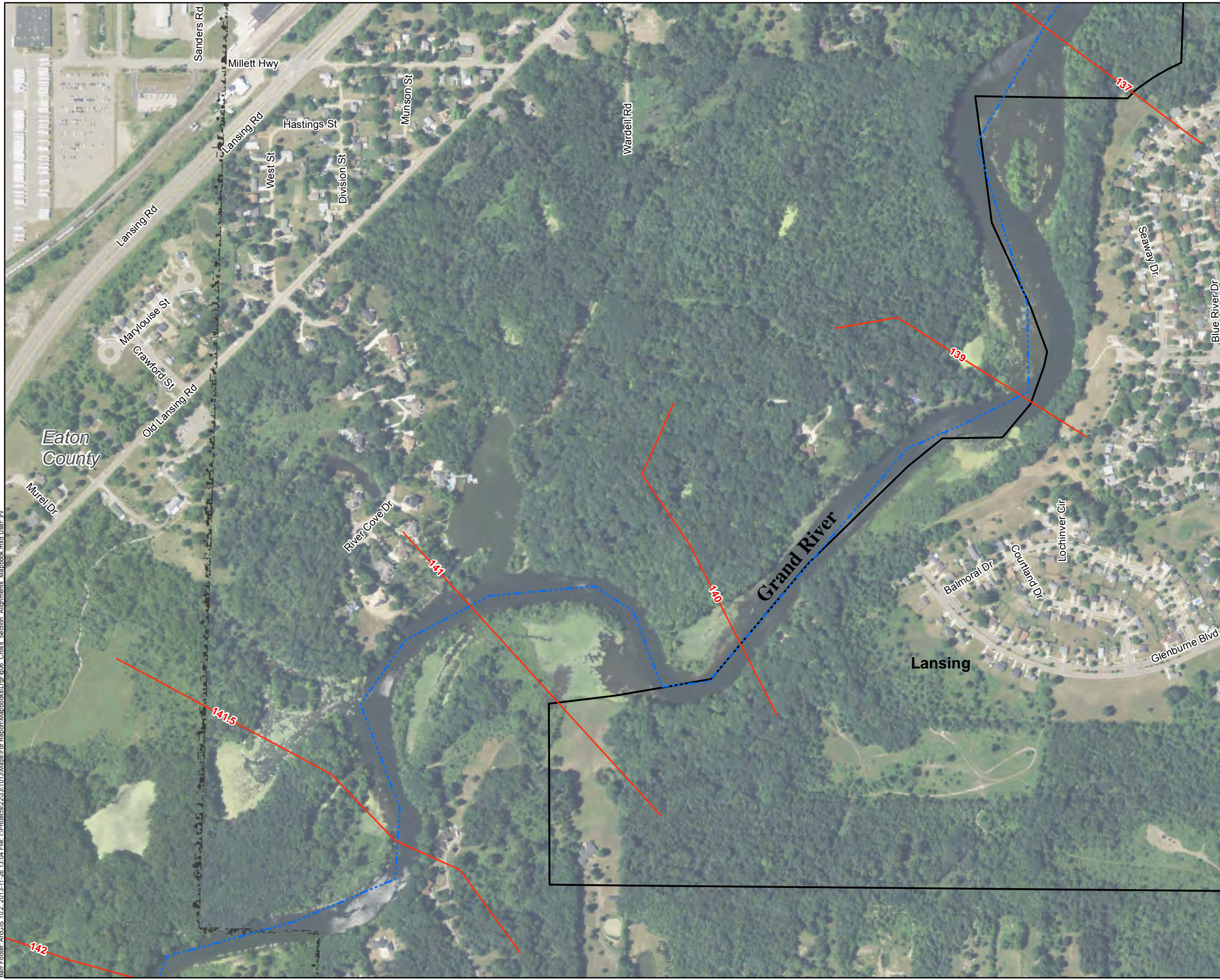
Large Figure 6 – 02 HEC-RAS CROSS SECTIONS Moores Park Dam and North Lansing Dam Break Model Lansing Board of Water and Light November 2013
