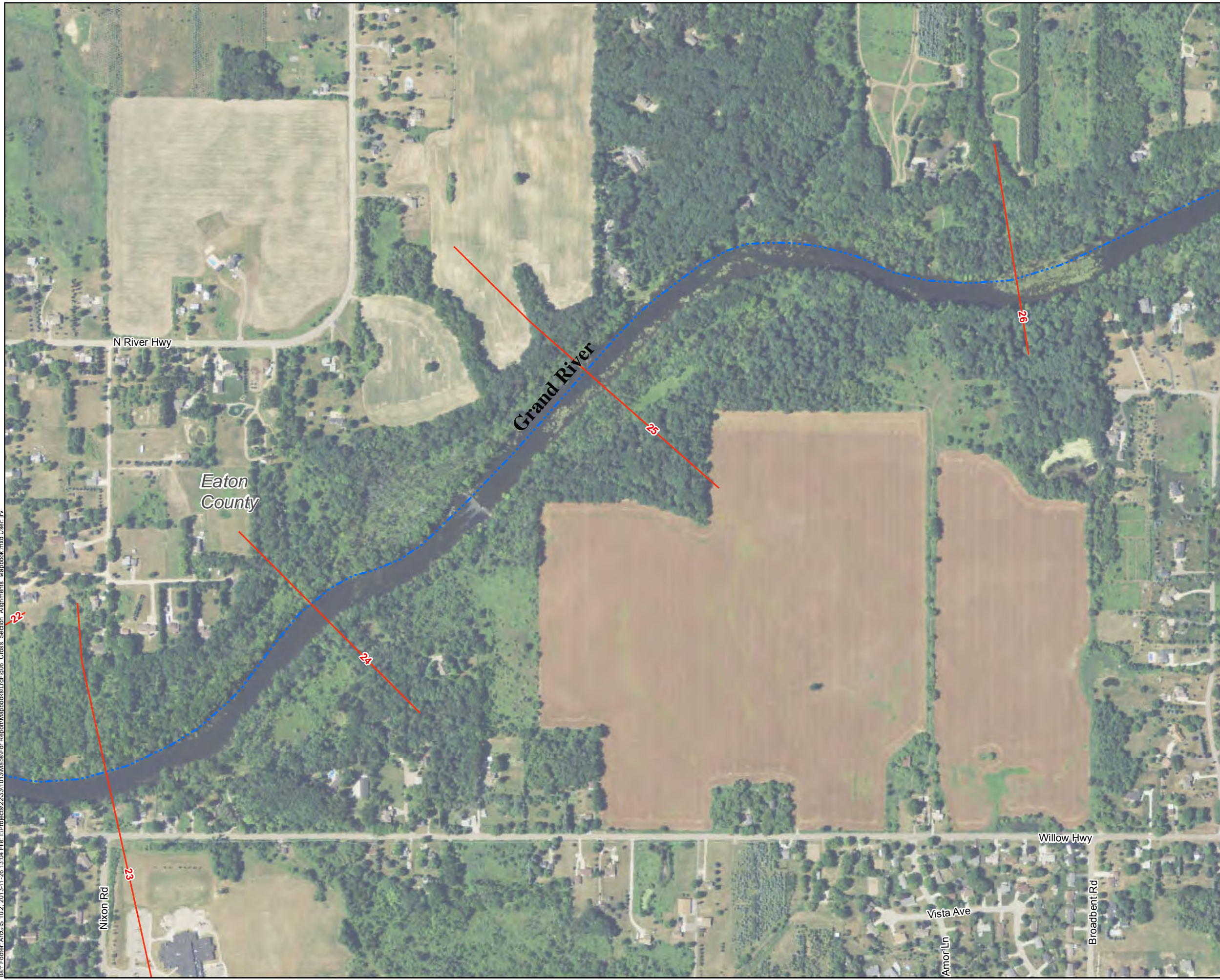
Large Figure 6 – 15 HEC-RAS CROSS SECTIONS Moores Park Dam and North Lansing Dam Break Model Lansing Board of Water and Light November 2013
